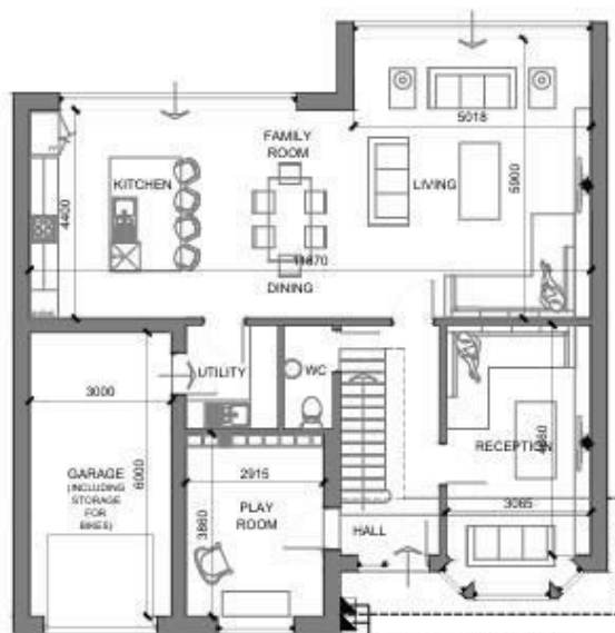
GROUND FLOOR PLAN 1:100 SCALE
